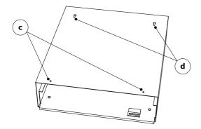
To install the cash drawer unit, use screw with heads that are as flat as possible to ensure the smooth movement of the sliding drawer.
