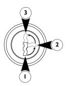
All cash drawer models (except 28E) can be locked or unlocked using a cylinder lock:
