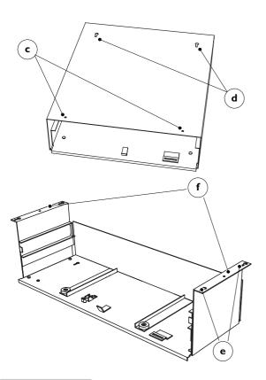
To install the cash drawer unit, use screws with heads that are as flat as possible to ensure smooth movement of the sliding drawer.
